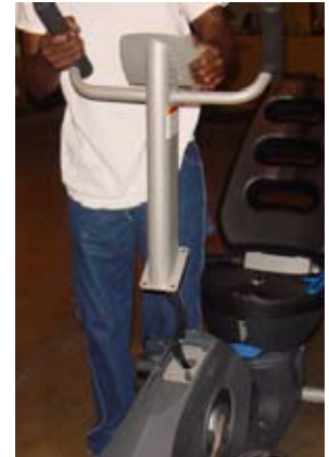
Figure 6b - Lift mast off frame (R916)
