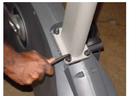
Figure 5a - Unbolt mast from frame (U916)
